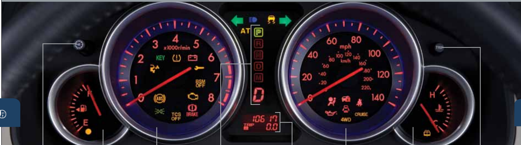
INSTRUMENT CLUSTER DIMMER 1 FUEL GAUGE TACHOMETER SHIFT LEVER POSITION INDICATOR ODOMETER/TRIP METER SPEEDOMETER ENGINE COOLANT TEMPERATURE GAUGE TRIP METER SELECTOR 2
