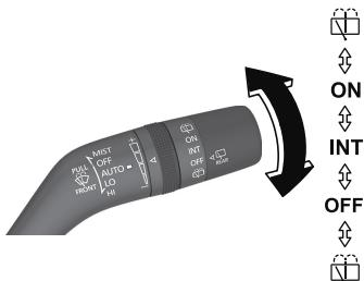
Turn the wiper on by turning the rear wiper/washer switch.
