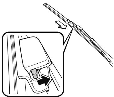
4. Pull the blade rubber in the direction of the arrow and slide it to a position where the blade holder groove can be checked.
