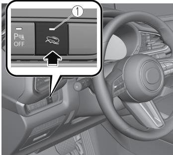
1. Off-Road Traction Assist switch indicator light
