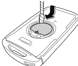
7. Insert a new battery into the transmitter so that the positive pole is facing up.
