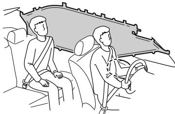
Only one side curtain air bag will deploy on the side of the vehicle that receives the force of an impact.
