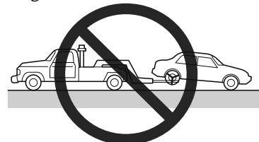
➤ Do not tow with sling-type equipment. This could damage your vehicle. Use wheel-lift or flatbed equipment.
