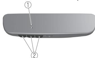
2. Hold the hand-held transmitter 2.5 to 7.5 cm (1 to 3 in) away from the HomeLink button you would like to program while keeping the indicator light in view.
