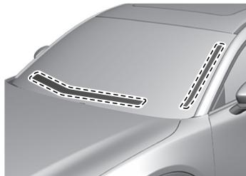
The windshield wiper de-icer operates in conjunction with the rear window defogger.
