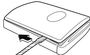
4. Twist the flathead screwdriver in the direction of the arrow and remove the upper cover.
