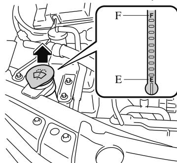
The top of the float should be between F and E.
