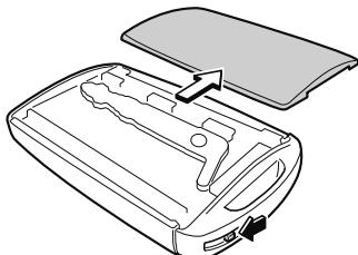
2. Remove the auxiliary key.
