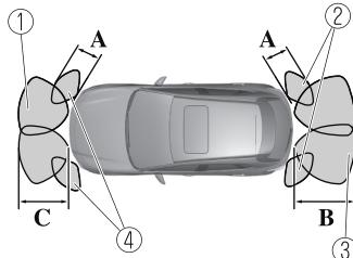
1. Front ultrasonic sensor detection range
