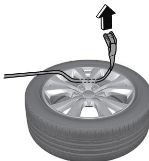
13. Thread the belt through the buckle, then pull the belt end to secure the flat tire.
