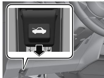
2. Insert your hand into the hood opening, slide the latch lever to the left, and lift up the hood.
