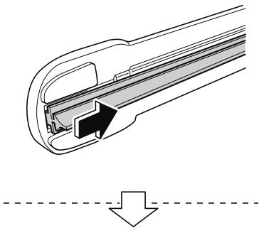
5. Pull the end of the blade rubber from the blade holder groove in the direction of the arrow and remove
