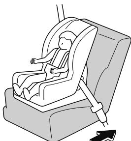
3. Remove the head restraint. However, when installing a backless booster seat, always install the vehicle head restraint to the seat
