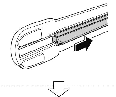
8. Make sure that the blade rubber is correctly installed to the blade holder.
