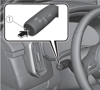
1. High beam control switch
