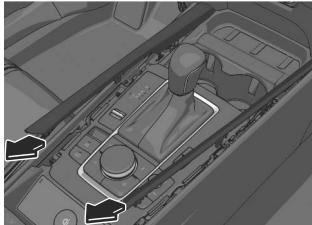
4. Lift the shift panel and detach the clips.
