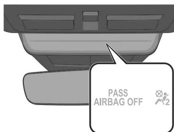
If the front passenger weight sensors are normal, the indicator light illuminates when the vehicle power is switched ON. The light turns off after a few seconds. Then, the indicator light
