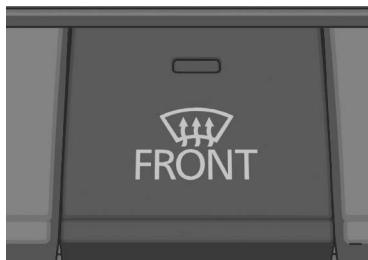
Switches the windshield defroster on (indicator light turned on) and off (indicator light turned off). Use to defrost the windshield and side windows.
