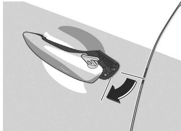
5. Attach the auxiliary key to its original position.
