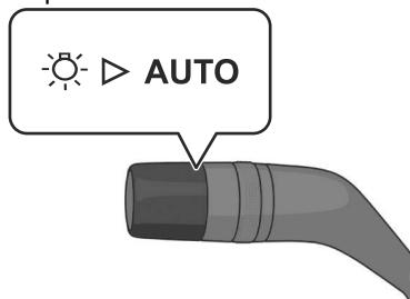
The daytime running lights turn on automatically when it is bright, and the headlights, parking lights, taillights, side-marker lights, and the license plate lights turn on automatically when it is dark.
