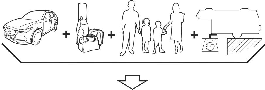
**GVW (Gross Vehicle Weight)** is the Vehicle Curb Weight + cargo + passengers.
