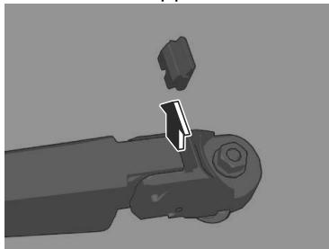
3. Raise the wiper arm and rotate the wiper blade to the right until it unlocks, then remove the blade.
