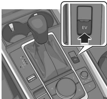
EV mode operates and the EV mode indication <sup>EV</sup> <sub>MODE</sub> turns on. Press the EV switch again to cancel EV mode.
