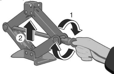
4. Place the jack under the jack-up position closest to the tire being changed with the jack head squarely under the jack-up point.
