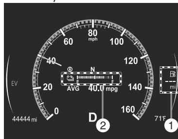
1. Maximum driving distance display for fuel and high voltage battery
