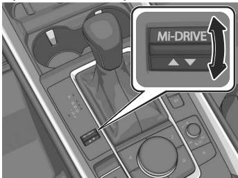
2. While checking the list displayed in the multi-information display, push the Mi-Drive switch forward or pull it toward you to select a drive mode.
