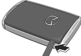
4. Twist the flathead screwdriver and remove the upper cover.
