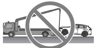
➤ If the parking brake cannot be released when towing the vehicle, transport the vehicle with all front and rear wheels raised off the ground as shown in the figure. If the vehicle is towed without raising the wheels off the ground, the brake system could be damaged.
