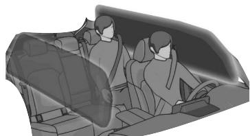
Both curtain air bags will deploy after the roll-over accident is detected.
