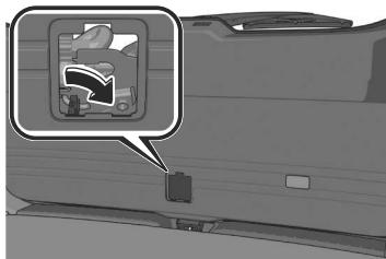
The liftgate is unlocked.
