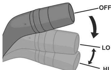
In the **LO** position, the windshield wipers operate at low speed. In the **HI** position, the wipers operate at high speed.
