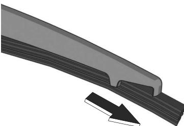
5. Remove the metal stiffeners from the blade rubber and install them in the new blade rubber.
