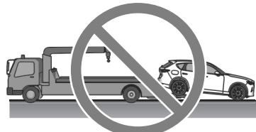
➤ Do not tow with sling-type equipment. This could damage your vehicle. Use wheel-lift or flatbed equipment.
