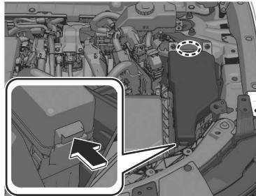
3. Open the cover for the booster battery terminal.
