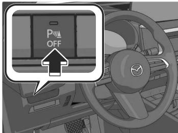
The parking sensors turn off and the parking sensor OFF switch indicator light turns on.
