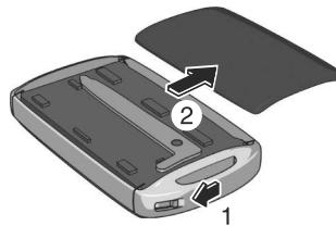
2. Press in the tab to unlock the upper cover.
