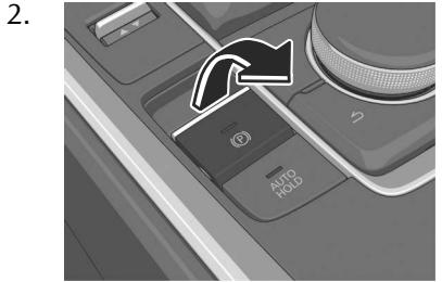
The parking brake is applied and the EPB indicator light <sup>(P)</sup> <sub>PARK</sub> in the instrument cluster and the EPB switch indicator light turn on.
