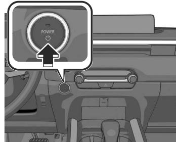
The hybrid system starts and the KEY indicator light (green)
