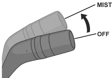
The windshield wipers operate while the lever is in the **MIST** position. Set the lever to the **MIST** position and immediately release it to operate the windshield wipers only once.
