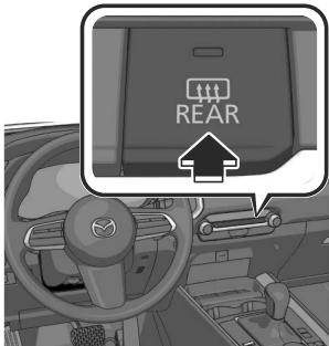
The rear window defogger operates and the switch indicator light turns on.
