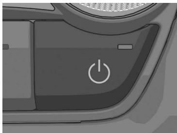
Switches the climate control system on and off.
