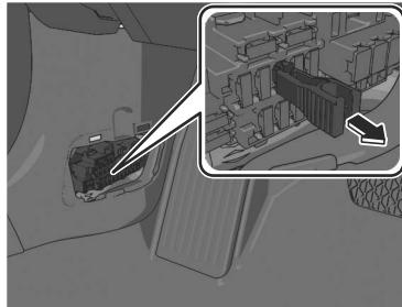
5. Inspect the fuse and replace it if it is blown.
