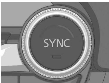
The mode switches between independent mode and interconnection mode each time the switch is pressed.
