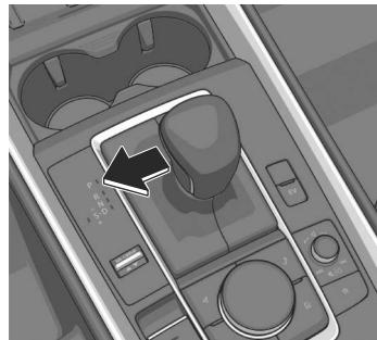
To return to automatic shift mode, shift the lever from S to D.
