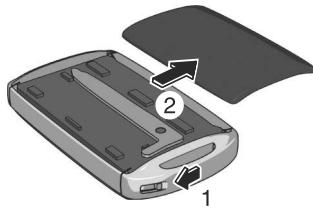
2. Remove the auxiliary key.
