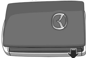
10. Attach the lower cover so that its tabs are inserted into the slots of the key.
