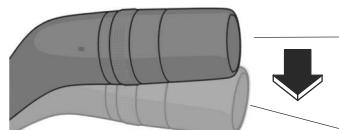
While the windshield wipers move out of their stowed positions to the point where they start reversing back, the washer fluid is sprayed and the wipers operate several times.
