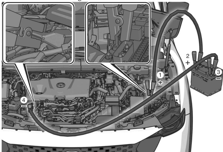
5. Start the booster vehicle's engine and rev the engine.
