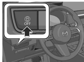
Press the i-ACTIVSENSE OFF switch to temporarily stop the following systems.
