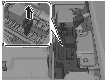
6. Inspect the fuse and replace it if it is blown.
