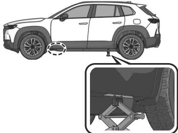
5. Continue raising the jack head gradually by rotating the screw with your hand until the jack head is inserted into the jack-up position.
