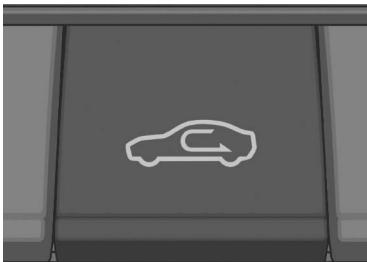
The mode is switched between recirculate mode and fresh air mode each time the switch is pressed. The display indicates whether recirculate mode (⟳) or fresh air mode (↔) is selected.
