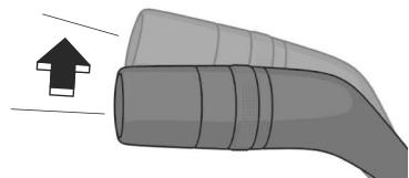
The headlights are switched to high beams and the headlight high-beam indicator light
