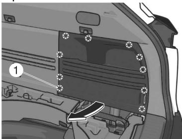
**Removing the Lead-acid Battery Cover**
