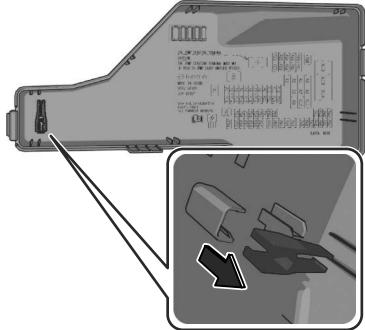
5. Pull the fuse straight out with the fuse puller.
