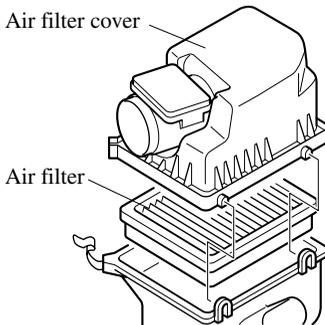
4. Wipe inside the air cleaner housing with a damp cloth.
