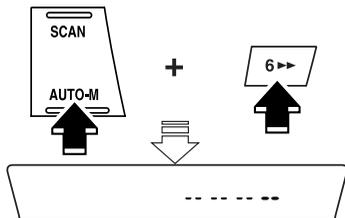
2. While the bars are displayed, input the code number as described in the setting procedure.
