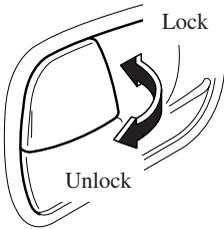
To lock any door with the door-lock knob from the outside, push the door-lock knob to the lock position and close the door.
