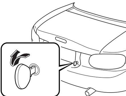
To activate the remote release, insert the key, turn it clockwise and open the trunk lid at the same time.
