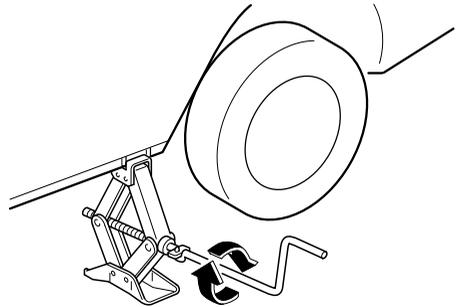
5. Remove the lug nuts by turning them counterclockwise; then remove the wheel.
