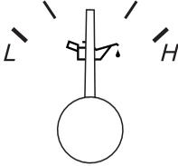
Engine oil pressure is normal when the engine oil pressure gauge needle points halfway between L and H with the engine running.
