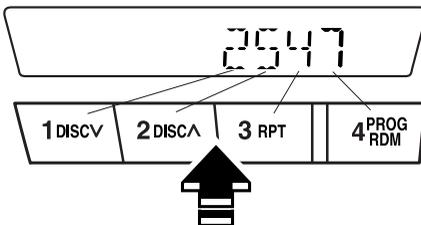
Press 1 for the first digit, 2 for the second, 3 for the third, and 4 for the last digit. For example, if your number is 2547, press 1 three times, 2 six times, 3 five times, and 4 eight times. If the display goes off while inputting, begin from Step 1.
