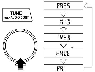
\*If your vehicle is not equipped with rear speakers, adjust the power/volume dial so level is even.
