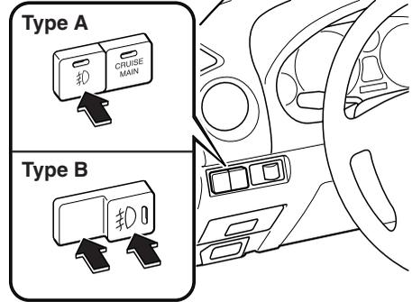
To turn on the fog lights, first turn the headlight switch to the position. Then press the fog light switch. To turn the fog lights off:
