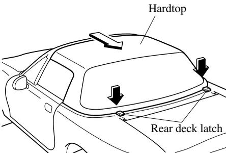
8. Lift the hardtop straight off the body to prevent damage to the rear deck latches and studs.
