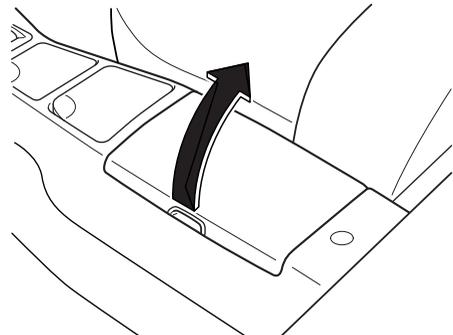
To release the trunk lid, pull up on the trunk lid release lever.
