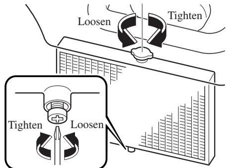
2. Only when the engine is cool, remove the radiator drain plug and drain the coolant into a suitable container. Properly dispose of the used coolant.
