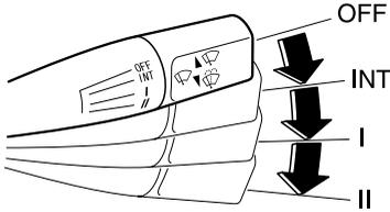
Turn the wipers on by pulling the lever down.
