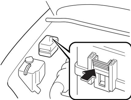
3. If a fuse is blown, replace it with a new one **of the same amperage rating**.
