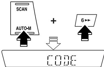
3. Again press the auto memory button (AUTO-M) and the channel preset button 6 simultaneously while "CODE" is displayed (within 10 seconds). The display will exhibit bars.
