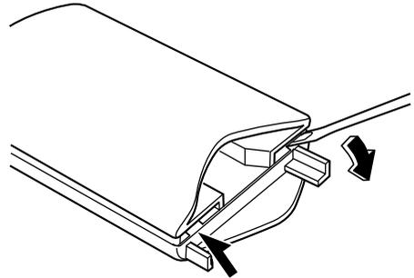
3. Press the portion of the battery indicated by A and remove the battery.
