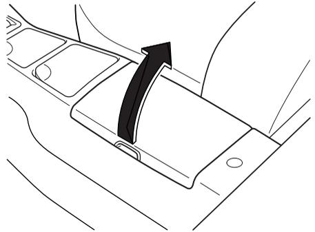
To open the fuel-filler lid, pull up on the remote fuel-filler lid release.
