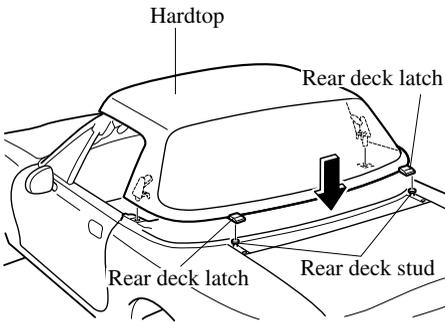
6. Slide the hardtop forward while pressing down on the rear deck latches to lock the latches, and then verify that they are secure by attempting to lift the rear of the hardtop.
