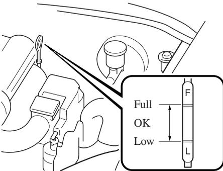
5. Pull it out again and examine the level. It's OK between L and F. But if it's near or below L, add enough oil to bring the level to F.
