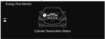
1. The condition of each cylinder is displayed by colors. The operating cylinders are displayed in red.
