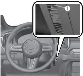
1. Interior temperature sensor
