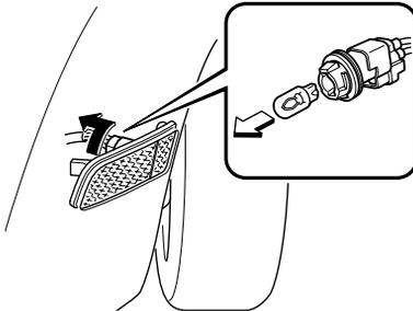
6. Install the new side turn signal unit in the reverse order of removal.
