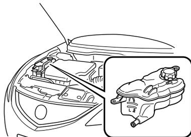
If it is at or near LOW or L, add enough coolant to the coolant reservoir to provide freezing and corrosion protection and to bring the level to FULL or F.
