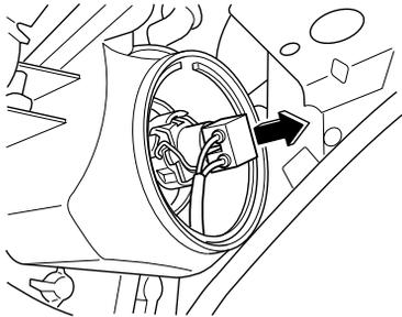
6. Unhook the bulb retaining spring.
